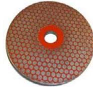
Grinder Disks - available in 180 standards, 260Grit fine and 360 extra fine Grit. Disks fit Diamond Max Grinders. Disks measure 5.875 diameter with a hole size .875 diameter Order Code:DMGD
